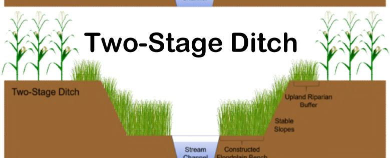
Two-Stage Ditches slow the flow of water and allow sediment and nutrients to settle on the benches before they enter the stream channel.
