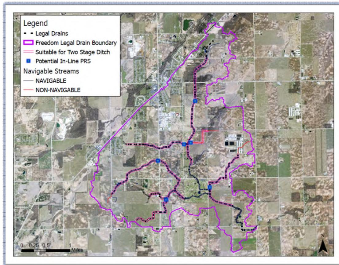
The above map of the Apple Creek Watershed identifies potential sites for Phosphorus Removal Systems (PRS) and two-stage ditches.
